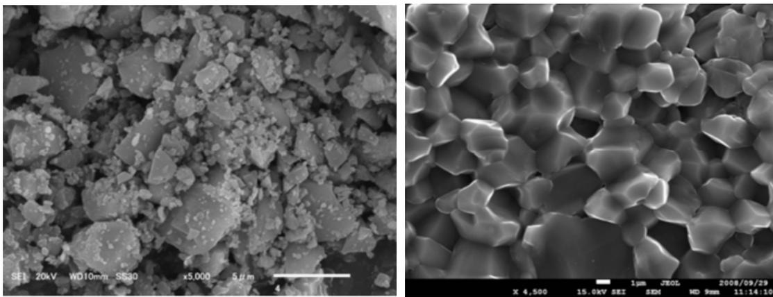
Figure 2. SEM images of the starting samples. Natural quartz powder; Min-U-Sil5 (left) and quartz aggregate; novaculite (right).
